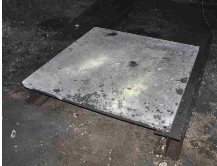
Figure 6.38. Panel B-5-P-2 after first detonation
