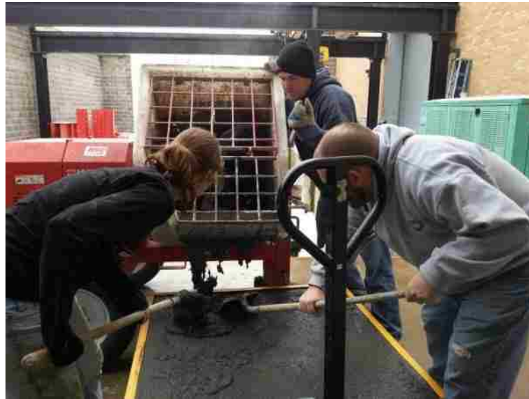
Figure 5.14. Panel specimen casting
