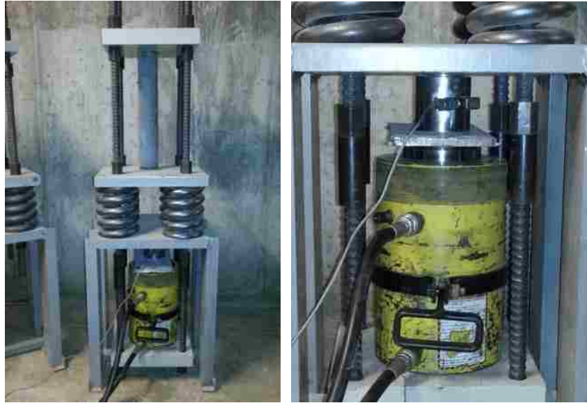
Figure 5.10. Loading of creep specimen
