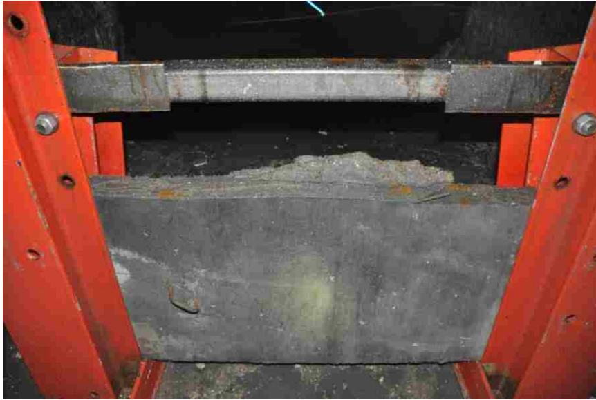
Figure 6.49. Back of H-2-6F-3.5 after detonation
