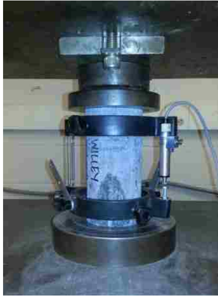
Figure 5.9. Modulus of elasticity test setup
