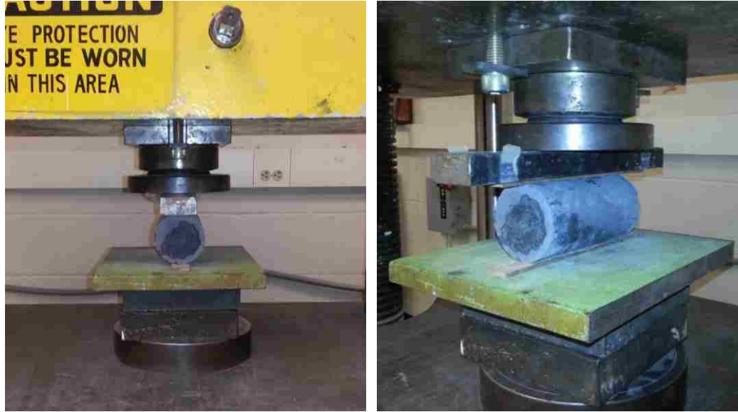
Figure 5.7. Splitting tensile test setup
