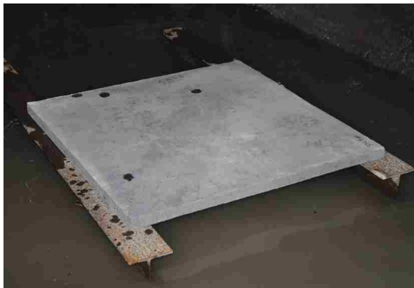
Figure 6.15. Panel B-4-2F-2 before detonation.
