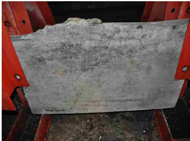
Figure 6.46. Front of H-2-6F-3.5 before detonation
