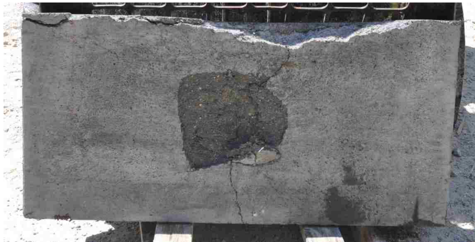
Figure 6.61. Tension face of panel H-7-6F-3.5 after detonation
