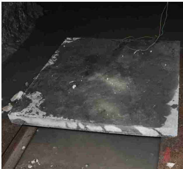
Figure 6.18. Top face of B-3-2F-3.5 after detonation
