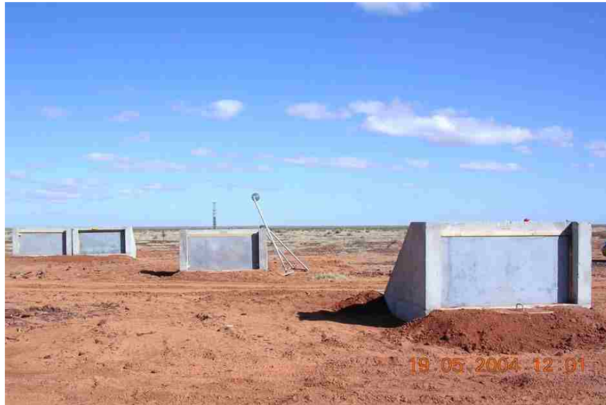
Figure 2.1. "Large-scale blast testing of Ductal protective panels at Woomera in 2004"
