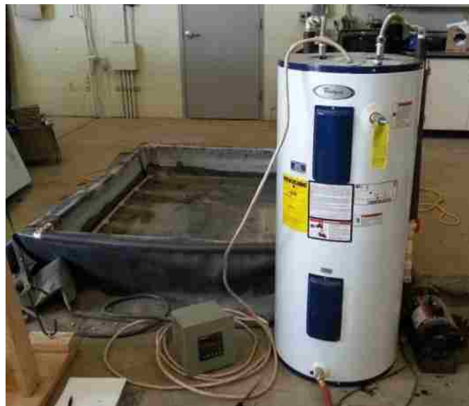
Figure 5.3. Full scale curing system
