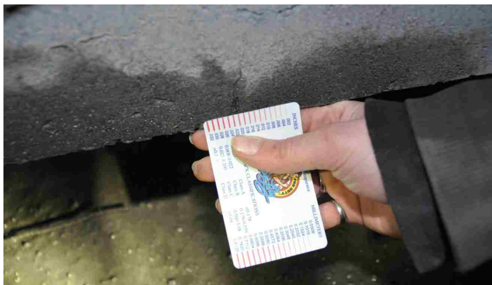
Figure 6.26. Crack development on front edge of B-1-6F-3.5 after first detonation
