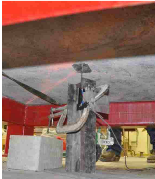
Figure 5.19. Linear potentiometer setup
