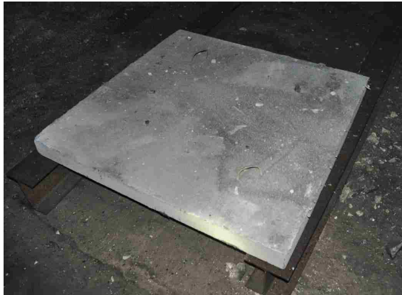
Figure 6.24. Top face of B-1-6F-3.5 after first detonation
