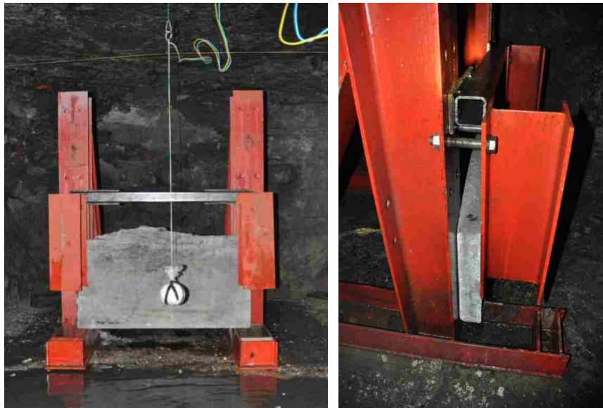
Figure 5.23. Half panel blast test setup
