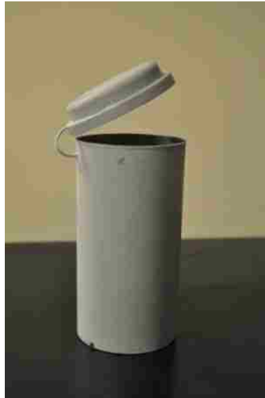
Figure 5.6. Splitting tensile specimen mold
