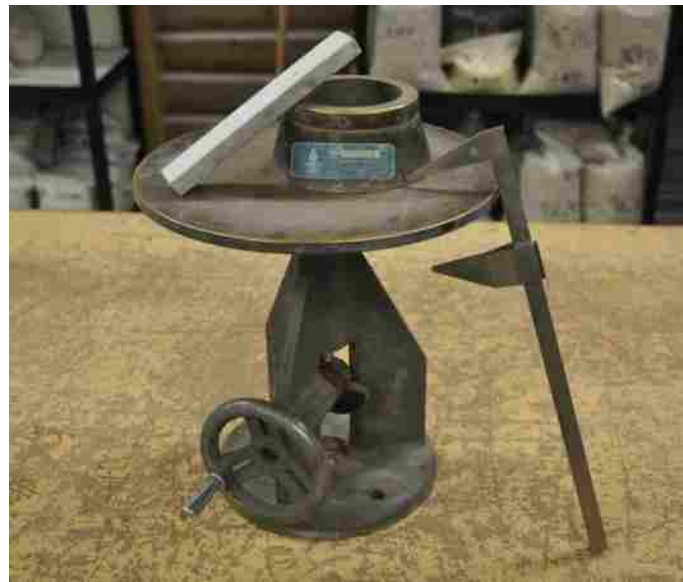
Figure 4.26. Flow testing equipment
