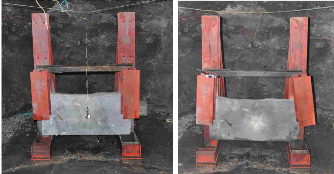
Figure 6.60. Panel H-7-6F-3.5 before (left) and after (right) detonation
