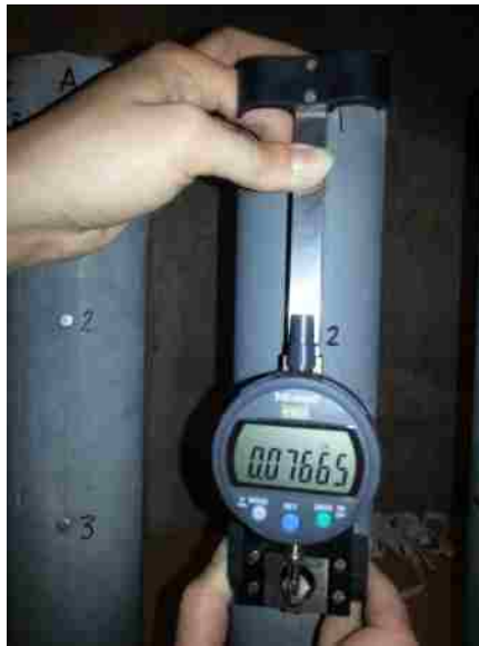
Figure 5.11. Sample strain gage reading
