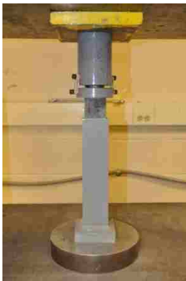
Figure 5.5. Compression test set-up
