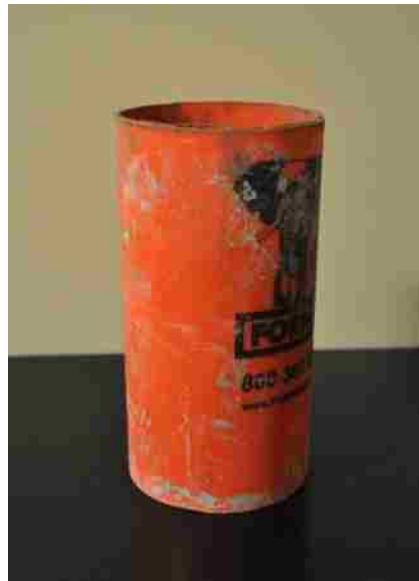
Figure 5.8. Modulus of elasticity specimen mold
