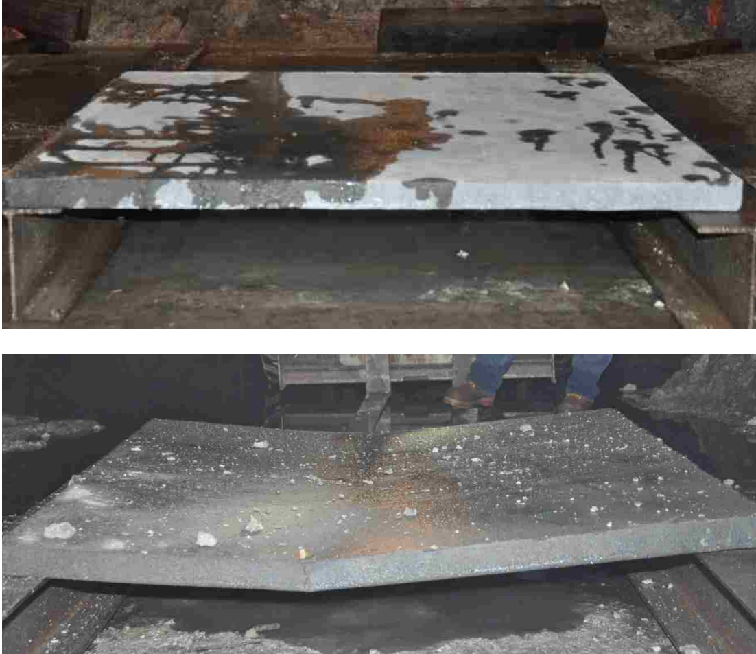
Figure 6.34. Deflection of B-6-6F-2 before (top) and after (bottom) detonation
