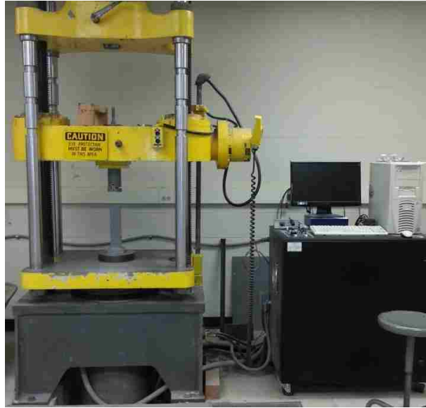
Figure 4.25. Mix trial compression test setup
