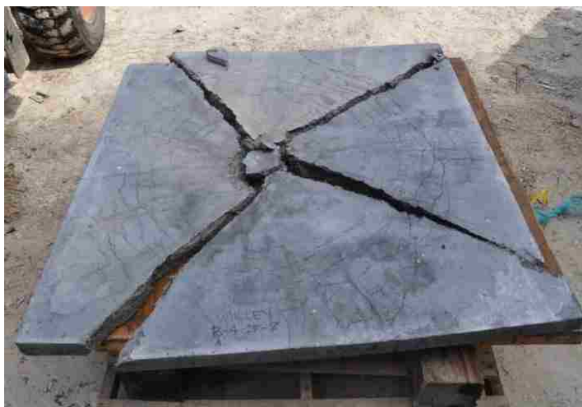
Figure 6.16. Panel B-4-2F-2 damage after detonation
