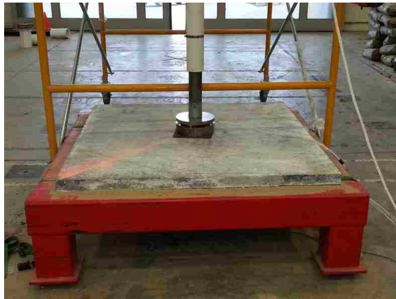
Figure 5.18. Impact test setup
