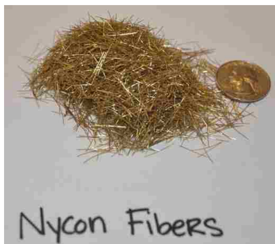
Figure 4.5. Nycon fibers used in small scale trials
