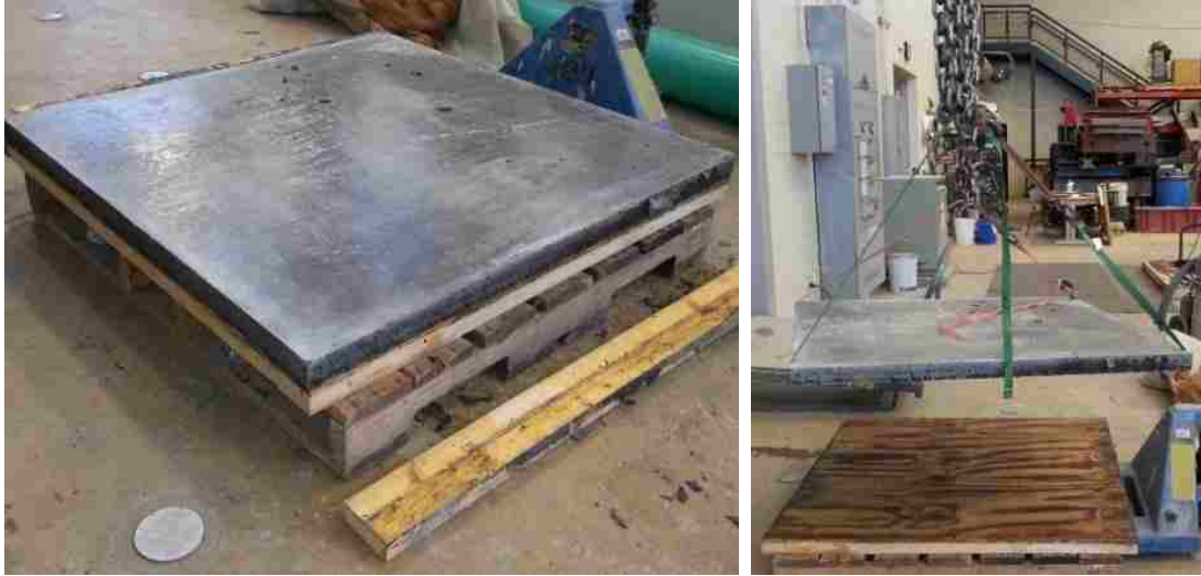
Figure 5.16. Panel de-molding process
