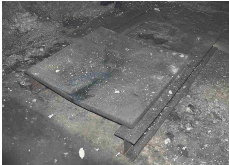
Figure 6.32. Top face of B-6-6F-2 after detonation
